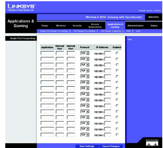
Figure 6-29 : Single Port Forwarding (Transfert de connexion unique)
